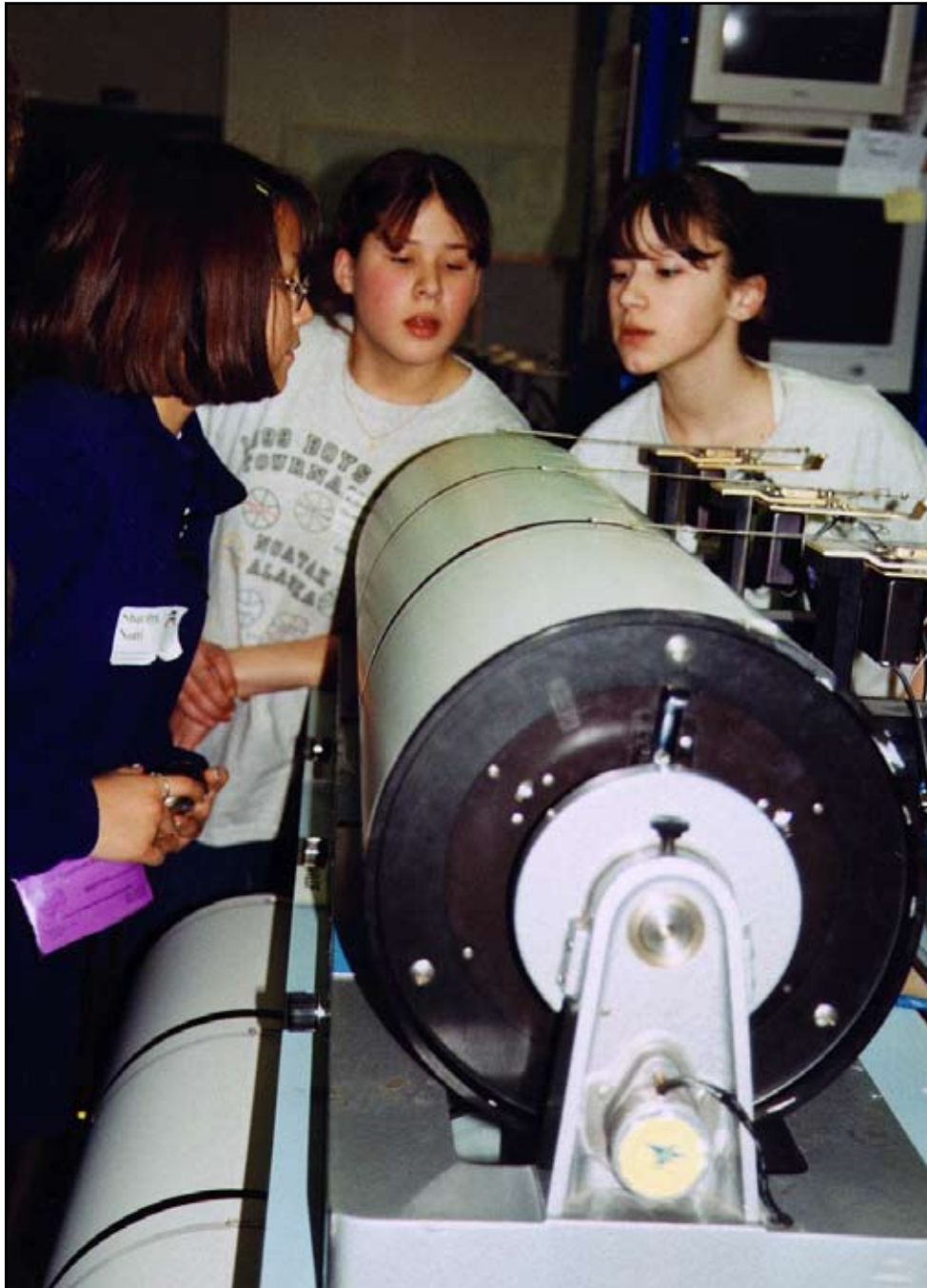
Middle-school students get a close-up look at the University of Alaska Fairbanks Geophysical Institute's seismograph array. The round drums shown above are seismographs.
