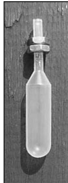
*The plastic eye dropper above has been weighted with two brass nuts to provide the added weight needed to sink the Cartesian diver.*
